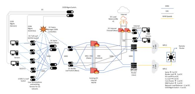
The upgraded 10G DC network connected with the existing 1G DC Network.
