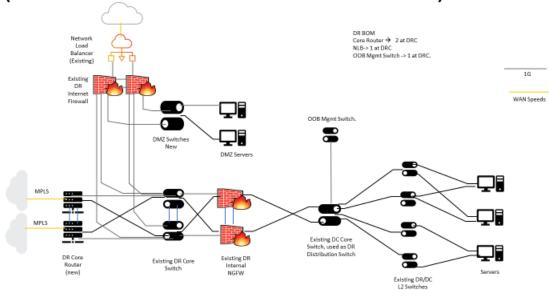
The DRC network would not be upgraded to SDN and would continue to be in the conventional Network System connected with the existing 1G DRC Network.
